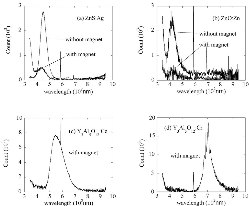
Fig. 2 Typical scintillation spectra from (a) ZnS(Ag), (b) ZnO(Zn), (c)  $Y_3Al_5O_{12}(Ce)$ , and (d)  $Y_3Al_5O_{12}(Cr)$ , with and without vertical field. (7 keV  $He^+$  beam bombardment)
