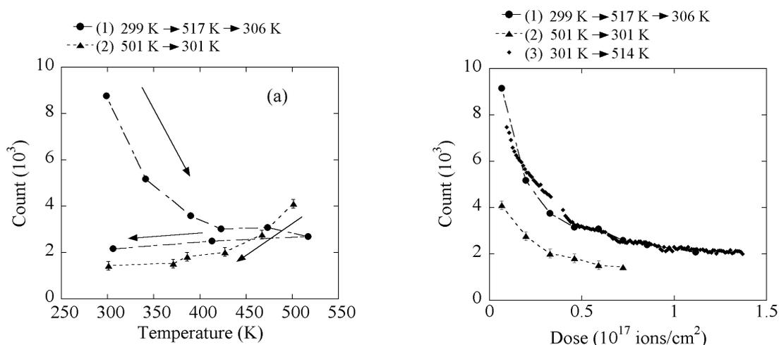
Fig. 3 Changes in scintillation efficiency of Y<sub>3</sub>Al<sub>5</sub>O<sub>12</sub>(Ce), (a) with temperature, and (b) with dose. (7 keV He<sup>+</sup> beam bombardment)
