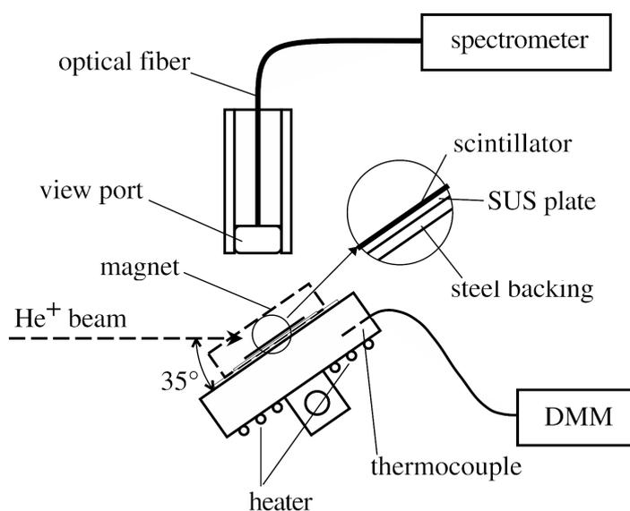
Fig. 1 Schematic view of the irradiation stage, with the scintillator holder, heater, thermocouple, a pair of permanent magnets to prevent electron bombardment, and a optical fiber coupled to a spectrometer.
