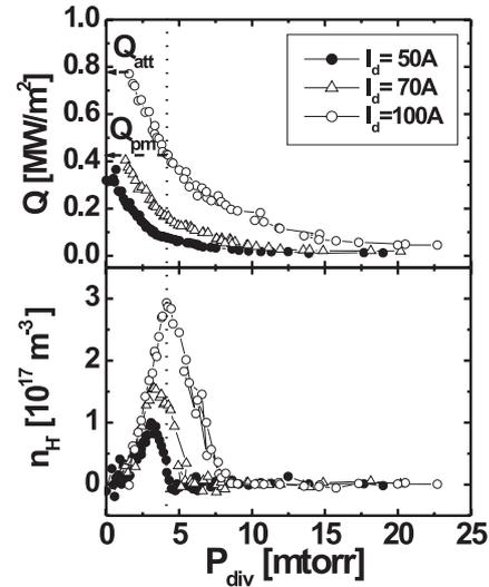
Fig.1 The variations of  $n_{H^- \text{ max}}$  and the heat load  $Q$  with the gas pressure  $P_{div}$ .
