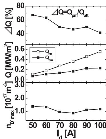
Fig.3 The variations of  $n_{D^- \text{ max}}$ , heat load  $Q_{att}$ ,  $Q_{pm}$ , and the heat load ratio  $\Delta Q$  with the discharge current  $I_d$ .
