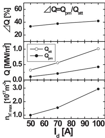
Fig.2 The variations of  $n_{H^- \text{ max}}$ , heat load  $Q_{att}$ ,  $Q_{pm}$ , and the heat load ratio  $\Delta Q$  with the discharge current  $I_d$ .
