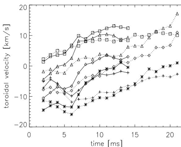
Figure 5: Rotation velocities of the  $n = -31$ ( $\square$ ),  $-25$ ( $\Delta$ ),  $-20$ ( $\diamond$ ),  $-15$ ( $*$ ) and  $-12$ ( $+$ ) tearing modes with (dotted) and without (solid) active feedback
