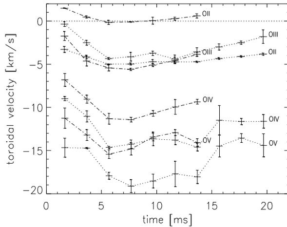
Figure 4: OII to OV toroidal velocities with (dotted) and without (dot-dashed) active feedback
