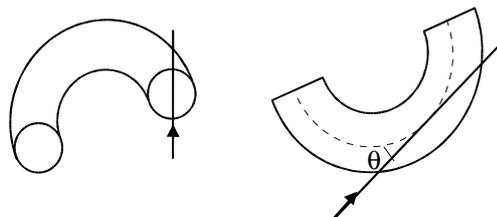
Figure 1: Lines-of-sight for zero velocity and toroidal velocity measurements respectively.
