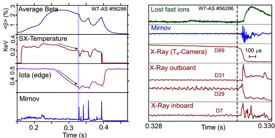
Fig. 1. Left: Dynamic change of the rotational transform by OH counter current drive ( $B = 1.25$  T). The electron temperature decreases towards low iota followed by several fast edge MHD bursts causing crashes of the plasma energy and termination of the current ramp. The crashes occur at the edge without precursors within about  $100 \mu\text{s}$  (right).
