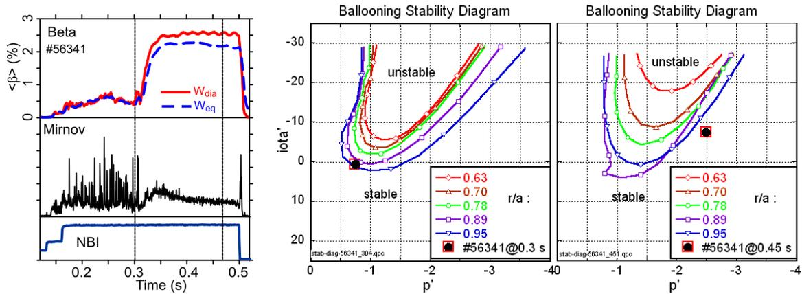
Fig. 4. Left: Spontaneous transition from an unstable low- $\beta$  phase into a quiescent high- $\beta$  regime in a configuration with enhanced modular ripple. The marginal stability contours (for different surfaces) are predicted for high- $n$  ideal ballooning modes [5]. The calculations indicate that the pressure profile is kept close to the 1<sup>st</sup> stability boundary in the first phase (middle). After the transition the second stability regime is reached (right).
