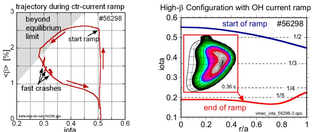
Fig. 2. Left: Evolution of beta as a function of the total edge transform in a discharge with an OH counter current ramp. As iota is ramped down, beta decreases keeping close to the estimated equilibrium limit where fast thermal crashes occur at a decreased temperature. Right: The current drive results in low iota with a flat profile. This is connected with a large Shafranov shift in the order of  $\Delta/a = 0.5$  as derived from X-ray tomography (inset).
