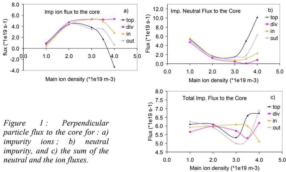
Figure 1 : Perpendicular particle flux to the core for : a) impurity ions ; b) neutral impurity, and c) the sum of the neutral and the ion fluxes.
