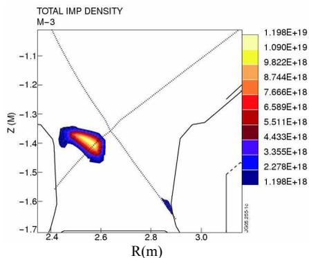
Figure 4: Total impurity density for the contour plot for the simulation with the highest power and main ion density.
