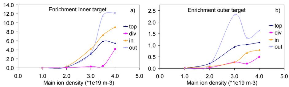
Figure 2: Enrichment as function of density for the four main ion puffing positions, divertor, top, inner mid-plane and outer mid-plane: a) inner target ; b) outer target.
