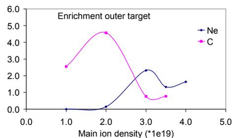
Figure 5: Enrichment for the outer target for the cases with a recycled impurity (Ne) and non recycled impurity (C).
