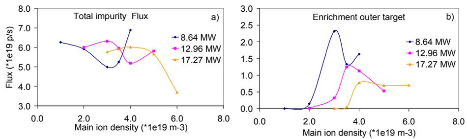
Figure 3: Total perpendicular impurity flux to the plasma core averaged along the seperatrix as a function of density for the different input powers, 8.64 MW, 12.96 MW and 17.28 MW when the top puffing was used. b) Enrichment.
