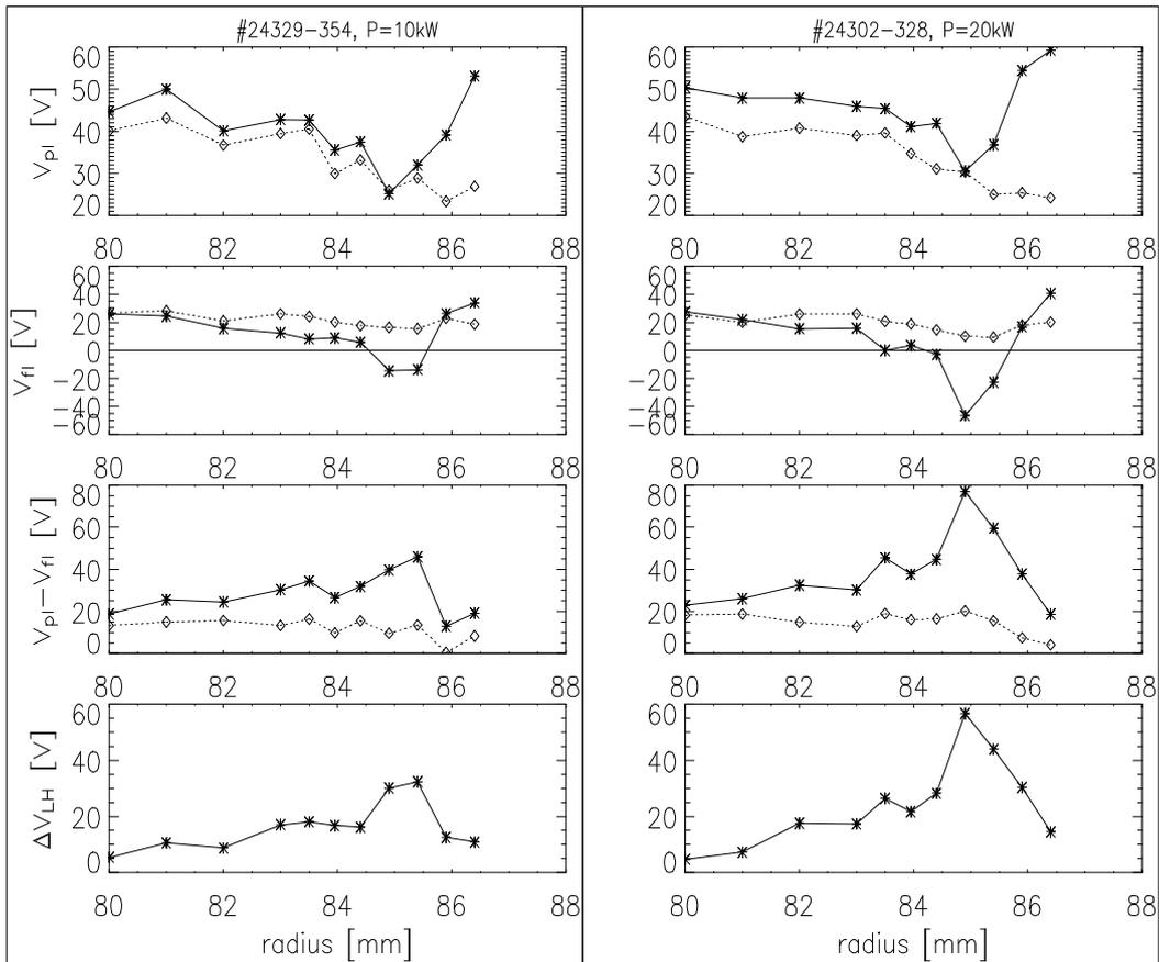
Fig. 1. Radial profiles of the emissive ( $V_{pi}$ ) and the cold ( $V_{fi}$ ) probe floating potentials in OH (diamonds) and LH (asterisks) discharge phase (left–10kW, right–20kW of LH power).
