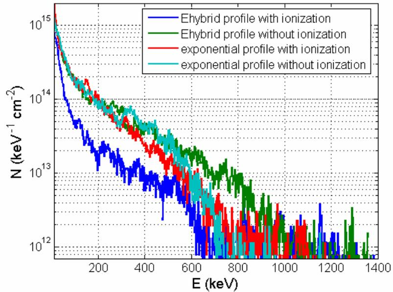
**Fig. 2:** Hot electron distributions calculated by PIC code with and without ionization. The results denoted by 'Ehybrid profile' start with the initial density profile denoted 'approximation' in Fig. 1. For comparison, we include the results calculated with only the exponential part of this profile. The parameters are: 45 fs, 800 nm, p-polarized laser pulse with intensity  $10^{17}$  W/cm<sup>2</sup> and angle of incidence 25°.
