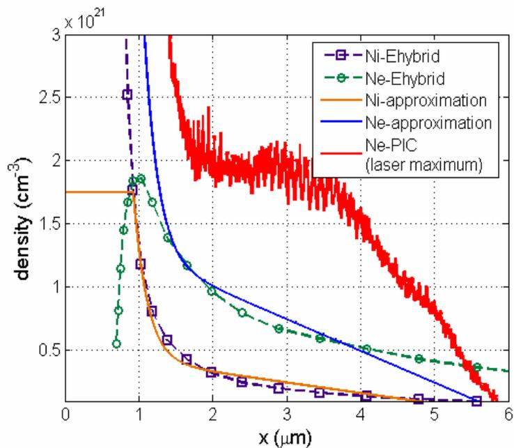
**Fig. 1:** The ion (Ni) and electron (Ne) plasma density profiles as calculated by Ehybrid code for 1 ns irradiation of Ag target by 800 nm,  $10^{10}$  W/cm<sup>2</sup> laser pulse and their approximations used in PIC simulation. The red electron density profile Ne-PIC is added to illustrate the evolution of electron density in PIC simulation of laser plasma interaction with ionization.
