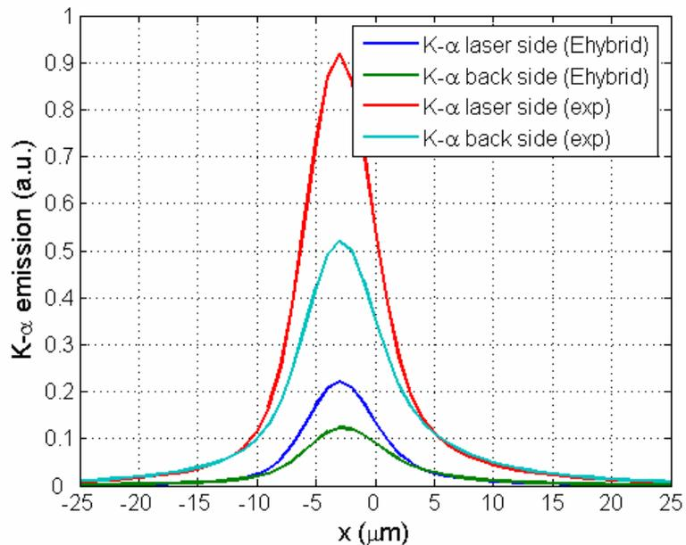
**Fig. 3:** K- $\alpha$  emission spot sizes calculated by our MC code with hot electrons resulting from PIC simulations. We denote 'Ehybrid' the hot electron distribution plotted in Fig. 2. with blue color and 'exp' the cyan one.
