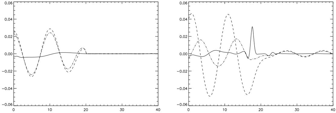
Figure 1:  $E_x$ ,  $E_y$  and  $B_z$  (full, dashed and dot-dashed line) vs.  $x$  for  $E_{y,dr} = 0.05$ ,  $\omega = 0.7$  at  $t = 20$  and  $t = 75$ , left and right frame, respectively.
