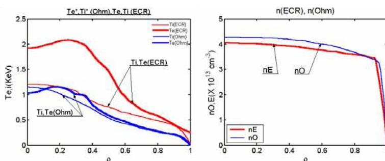
**Fig. 1a, 1b.** Radial distributions  $T_e$ ,  $T_i$  and  $n$  in regimes with "H-mode" regimes for cases of initiation of transitions at ECH and ohmic heating.
