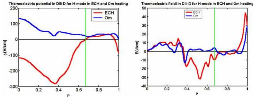
**Fig. 2a, 2b.** Radial distributions  $\varphi$ , and  $E_r$  in “H-modes” regimes for cases of initiation transitions by means of ECH and ohmic heating.
