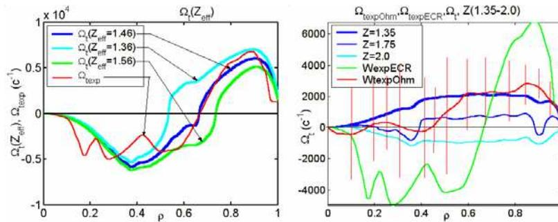
**Fig. 3a, 3b.** Radial distributions of rotation of plasma on DIII-D in "H-modes" regimes for cases initiation of transitions by means of a) ECH and b) ohmic heating.
