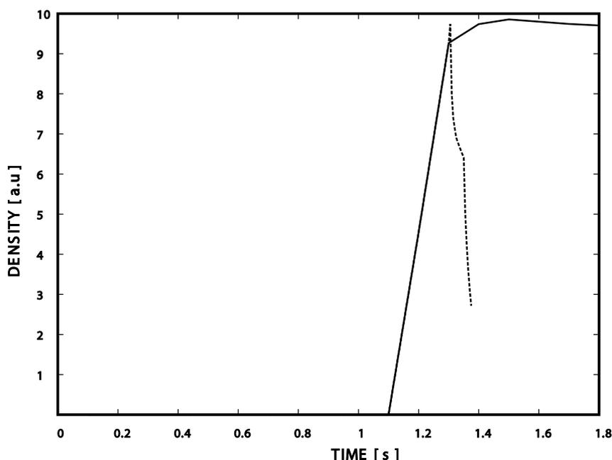
Figure 4: The time evolution of the total argon concentration in case density ratio  $n_H/n_D = 0.47$ : without ripple losses (solid line), with ripple losses (dash line)
