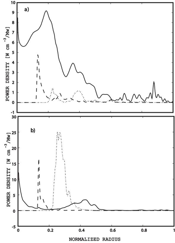
Figure 3: The radial profiles of absorbed power by electrons (solid line),  $\text{Ar}^{15+}$  (dash line),  $\text{Ar}^{16+}$  (dot line). Case a)  $n_H/n_D = 0.69$ , b)  $n_H/n_D = 0.47$
