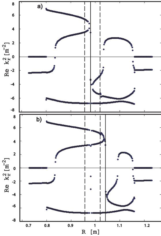
Figure 2: The radial profiles of  $k_{\perp}^2$  for different concentration ratio a)  $n_H/n_D = 0.69$ , b)  $n_H/n_D = 0.47$
