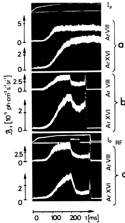
Figure 1: Time evolution of radiance  $\mathcal{B}_z$  of  $\text{Ar}^{7+}$  and  $\text{Ar}^{15+}$ : a) Ohmic discharge b) RF pulse on  $n_H/n_D = 0.685$  c) RF pulse on  $n_H/n_D = 0.485$ . Data from Ref. [1]
