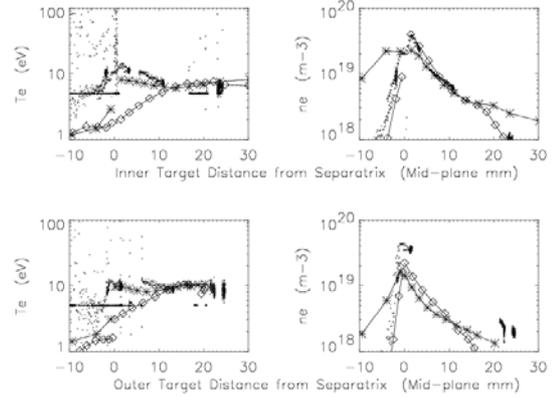
Figure 2. Inner (top) and outer (bottom) target  $T_e$  (left) and  $n_e$  (right) profiles as measured by the Langmuir probes (points), simulated by EDGE2D (stars) and by SOLPS5 (diamonds) for shot number 59733, REV-B.
