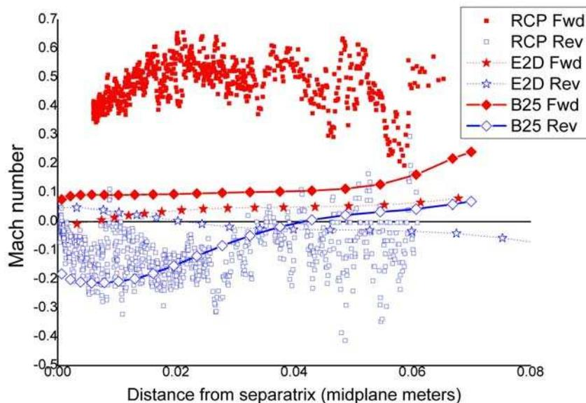
Figure 3. Comparison of Mach number profiles from RCP data (RCP: points), EDGE2D (E2D: stars) and SOLPS5 (B25: diamonds) simulations. FWD-B: filled symbols, REV-B: hollow symbols.
