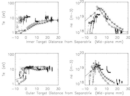
Figure 1. Inner (top) and outer (bottom) target  $T_e$  (left) and  $n_e$  (right) profiles as measured by the Langmuir probes (points), simulated by EDGE2D (stars) and by SOLPS5 (diamonds) for shot number 56725, FWD-B.
