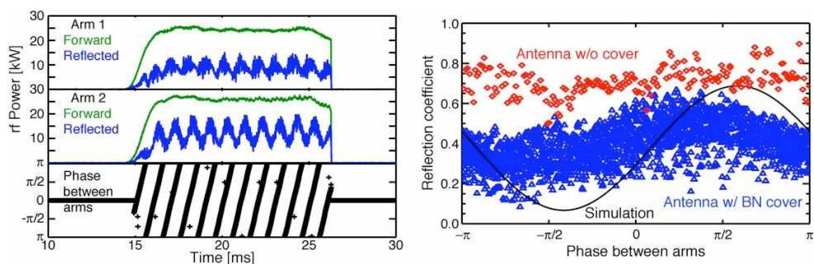
FIGURE 2. Tests of a twin-waveguide antenna designed to launch waves to couple to the EBW have been performed on MST. The reflected power in each waveguide changes with the applied phase between arms. The optimal phase has been determined and compared to that calculated from full-wave theory. The slight difference in optimal phase may be due to the boron nitride antenna cover.
