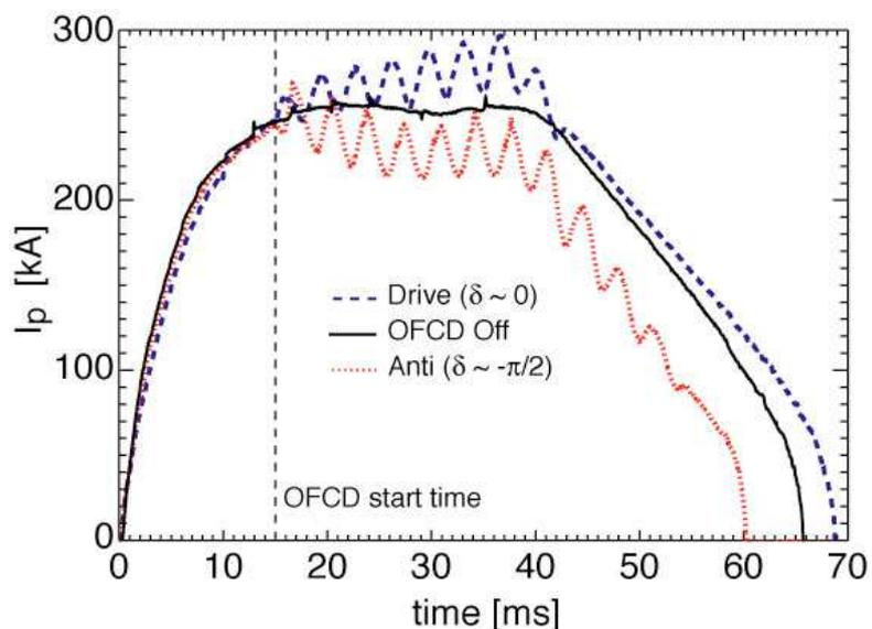
FIGURE 4. OFCD has been used to drive up to 10% of the plasma current in MST. Phase scans have been performed to determine the optimal phase between oscillators for maximum and minimum current drive. The amount of current driven does not increase with baseline current. Magnetic field penetration has been measured during OFCD. A rich variety of MHD effects, including sawtooth entrainment, mode amplitude changes, and ion heating, have been seen and are under active investigation.
