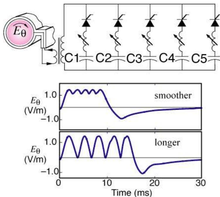
FIGURE 3. Diagram of the upgrade to the poloidal electric field circuit used for PCD on MST. The addition of variable inductors allows for the choice of a longer or smoother  $E_\theta$  waveform. A design for active control of  $E_\theta$  using programmable power supplies is underway.
