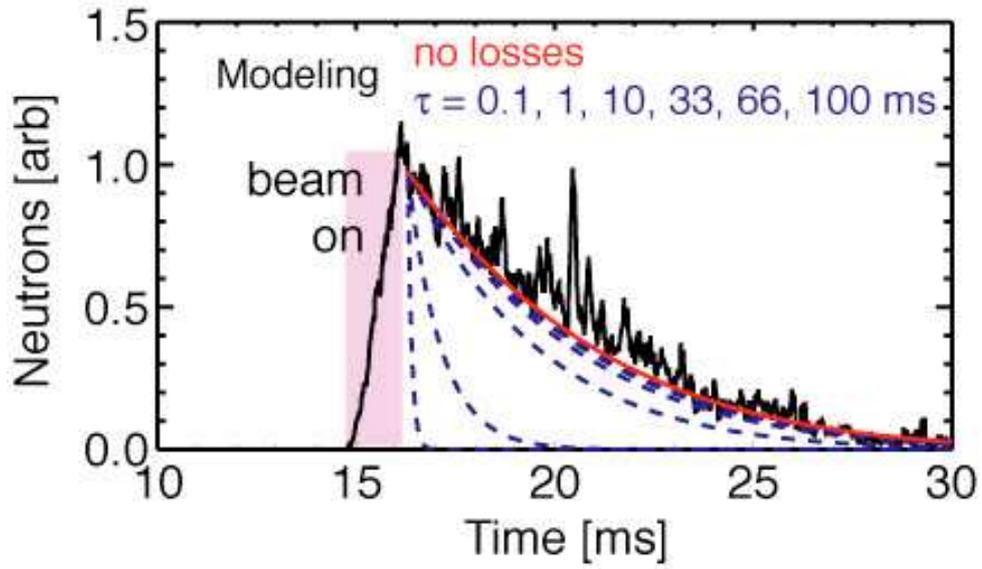
FIGURE 5. Neutrons generated from beam-plasma interactions are measured during neutral beam operation on MST. The fast ion confinement time inferred using modeling of the slowing down time and the fusion cross section is good:  $\tau \geq 30$  ms. Fast ion confinement studies are ongoing as are plans to upgrade to a long pulse neutral beam suitable for heating and current drive experiments.
