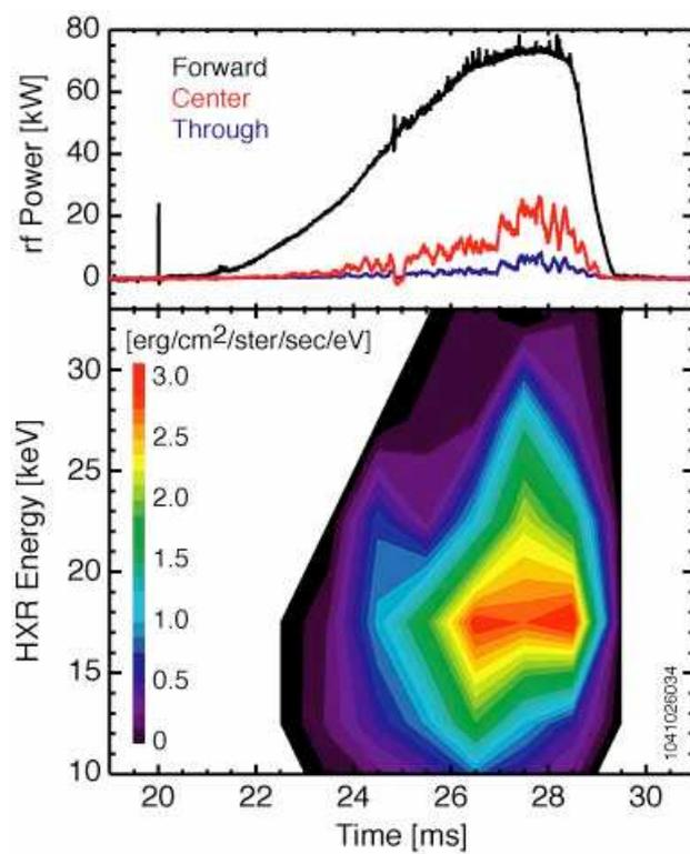
FIGURE 1. Hard x-rays up to 25 keV in energy are observed during lower hybrid wave injection on MST. The x-ray production is best correlated with rf propagation along the antenna. HXRs are measured when power flows in either direction through the antenna.
