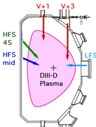
Fig. 1 Cross-section view of DIII-D showing the pellet injection locations.
