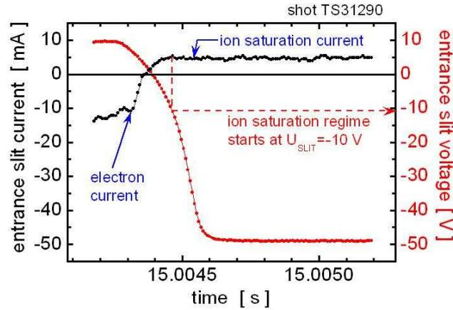
Fig. 2. RFA entrance slit current in ohmic regime, no LH power launched.
