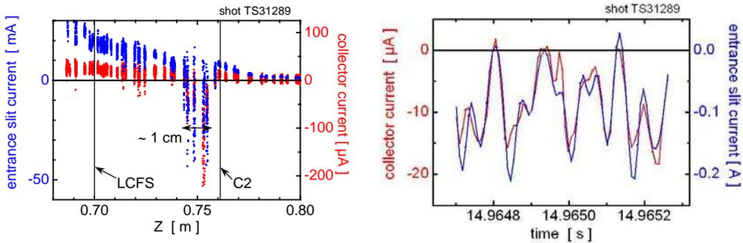
Fig. 3. a-left panel: A more detailed structure of the negative peak as seen in Fig.1, plotted as a function of the vertical RFA position. b-right panel: Detailed temporal structure of the peak of the negative current.
