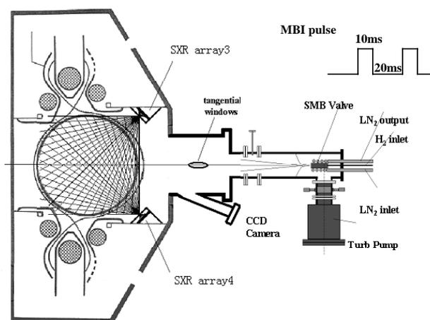
Fig. 1. Arrangement for MBI in the HL-2A tokamak.
