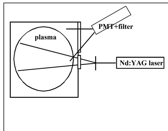
**Fig. 2.** Sketch of the experimental set-up devised to explore the proposed dust detection scheme.
