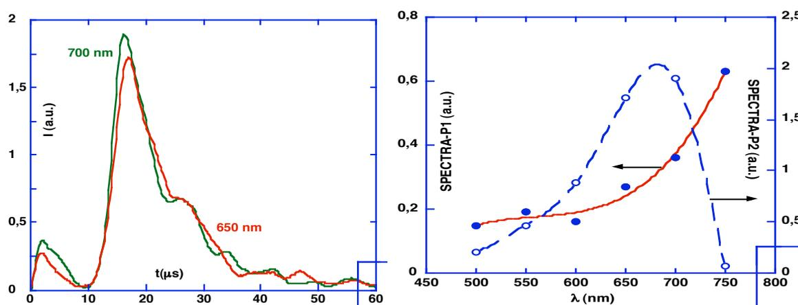
**Fig. 3.** Results of a dust-simulation-experiment using the TJ-II laser blow-off injection system. Here: left) is the time evolution of the signal at two wavelengths; right) is the spectral shape of the two separate temporal peaks: the first peak is identified as a dust by-product effect.
