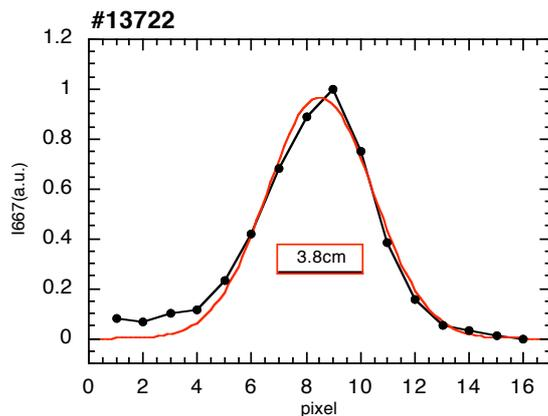
Figure 2. The recorded toroidal profile of 667nm line (11.2cm span) shows a beam FWHM when it propagates into the plasma. This is  $\sim 2x$  the beam width in vacuum.
