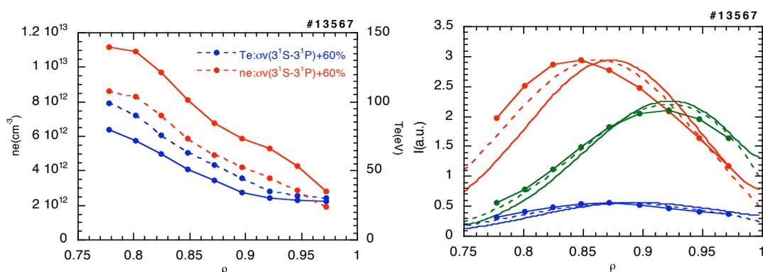
Figure 1. Density and temperature profiles obtained by the C-R model and by the same model using a 60% higher value of the  $3^1\text{S}-3^1\text{P}$  transition rate coefficient (left). Experimental and simulated lines intensity profiles corresponding to both couple of profiles (solid and discontinuous lines respectively) on the right.
