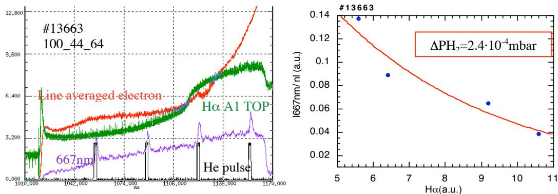
Figure 3 Attenuation of the He beam with the molecular neutral density.
