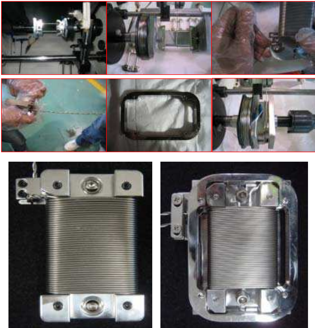
Fig. 3. Fabrication procedures and fabricated B_r and B_r+B_z probes.
