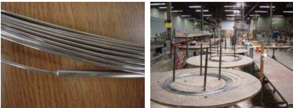
Fig. 2. Fabricated combined MgO insulated coaxial cables.
