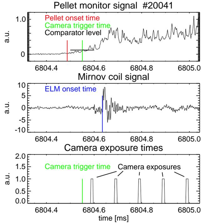
Fig. 1. The time evolution of the pellet monitor signal, the Mirnov coil signal and the camera exposure times. For the definition of the different time markers refer to the text.
