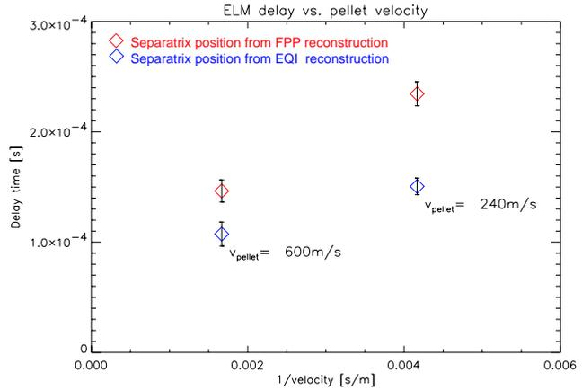
Fig. 4. The mean value of the delay between the ELM onset and the time when the pellet crossed the separatrix as a function of the inverse velocity.
