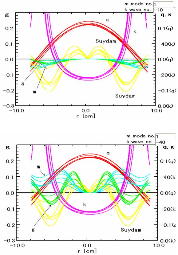
fig.3.  $W(\xi)$  integrated from the magnetic axis to  $r$ , safety factor  $q(r)$ , Suydam's condition and  $g(r)$  for  $m = 1$ ,  $k = -10$ (top) and  $k = -40$ (bottom).
