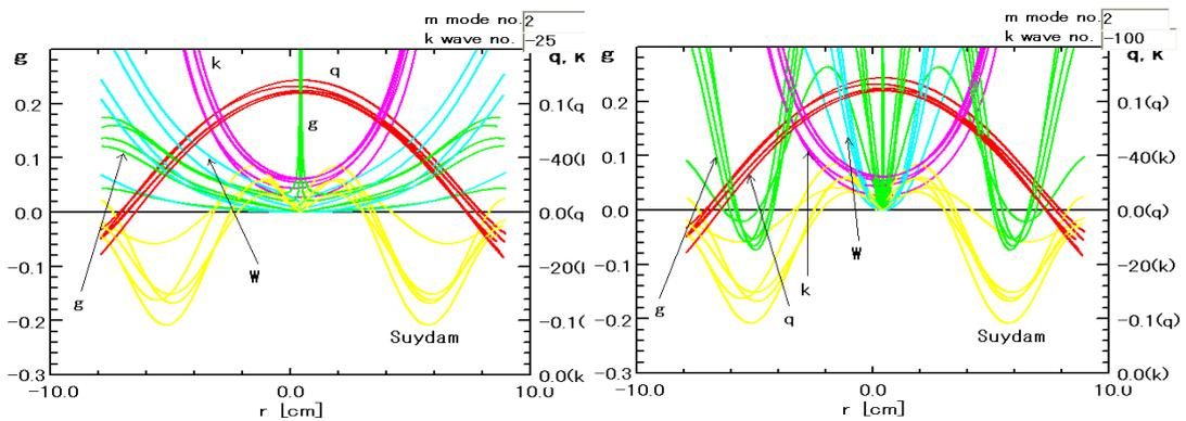
fig.4.  $W(\xi)$  integrated from the magnetic axis to  $r$ , safety factor  $q(r)$ , Suydam's condition and  $g(r)$  for  $m = 1$ ,  $k = -25$ (left) and  $k = -100$ (right). Pink line show the  $k$  value satisfying the  $krB_z + mB_\theta = 0$ .
