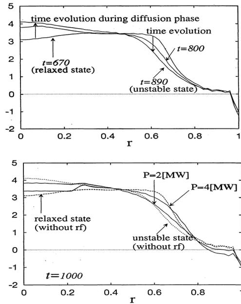
Fig. 2 The upper shows the time evolution of  $J \cdot B/B^2$ -profile during diffusion phase without rf-driven current, and the lower shows the comparison of  $J \cdot B/B^2$ -profiles between in the relaxed state without rf-driven current and in the stationary state with rf-driven current.
