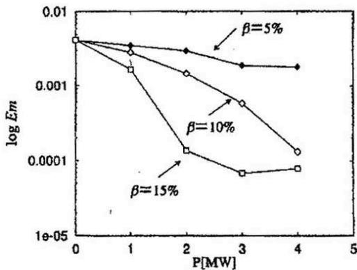
Fig. 3 Kink mode damping as function of rf power for each  $\beta$  value.
