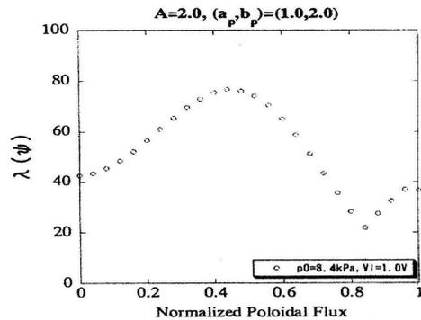
Fig. 4  $\lambda$ -profile as function of normalized poloidal flux in the neoclassical RFP equilibrium.
