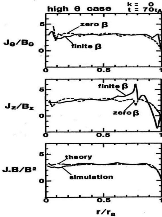
Fig. 1 The radial profile of the ratio  $J_\theta/B_\theta$ ,  $J_z/B_z$  and  $J \cdot B/B^2$  for zero  $\beta$  (dotted line) and finite  $\beta$  (solid line) simulations. The dot-dashed line is the predicted line by partially relaxed state model.
