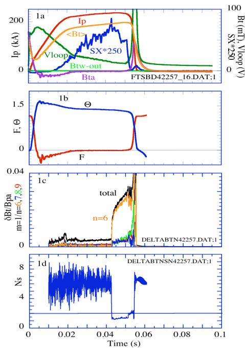
Fig.1 Discharge with the reproducible QSH state obtained by a very shallow reversal of  $B_{ta}$  ( $\sim 0$ ).
