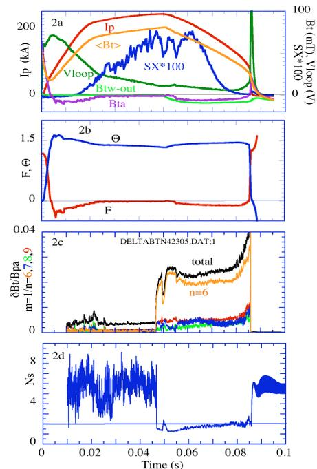
Fig.2 Discharge with prolonged QSH state by  $B_{ta}$  reversal ( $\sim 10mT$ ) with a delayed trigger (at 50ms).
