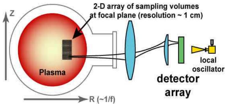
Fig. 2: Schematic representation of the ECE-Imaging system.
