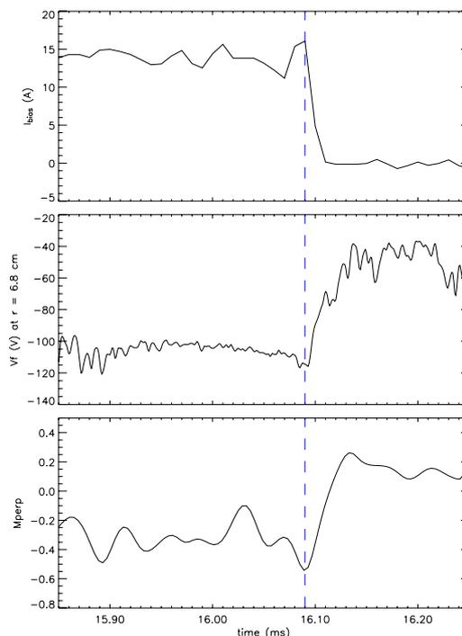
Fig. 4 - Plasma parameters during bias switch off.
