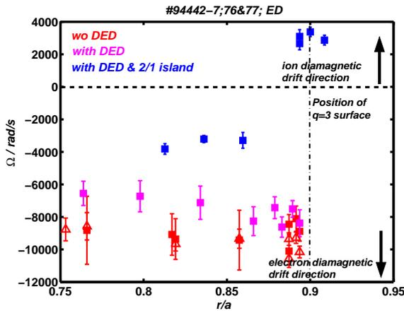
Figure 1: Turbulence rotation estimated in 3/1 configuration.
