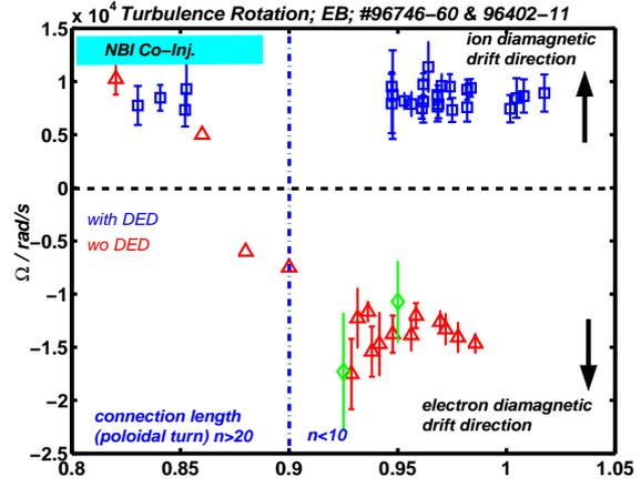
Figure 2: Turbulence rotation in 12/4 configuration. In addition  $\Omega_{\Theta}$  estimated from Doppler shifted carbon ions is shown in green
