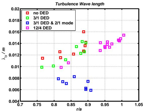
Figure 5: Estimated  $\langle \lambda_\Theta \rangle$  from autocorrelation function. The locked 2/1 mode during 3/1-configuration yields to a reduction of  $\langle \lambda_\Theta \rangle$  which is an indication of a reduced transport
