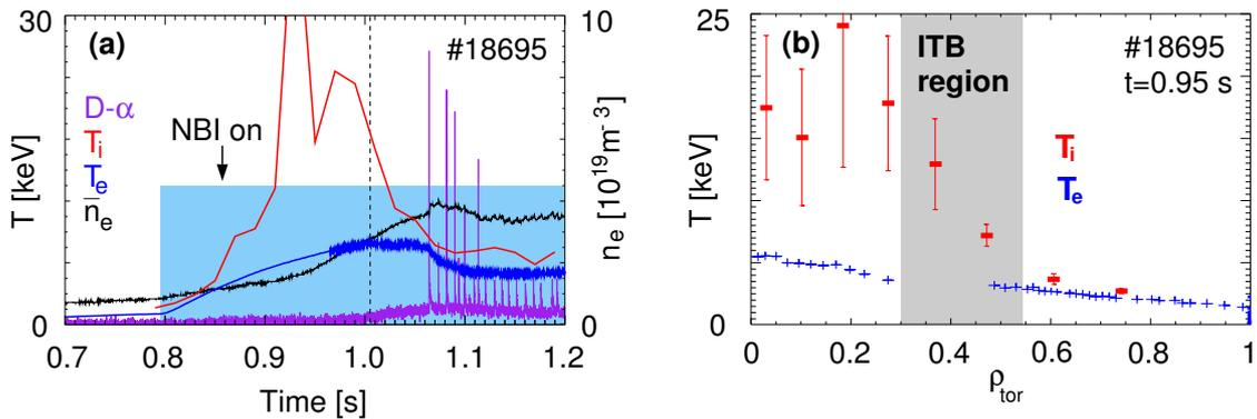
**Figure 1.** Discharge #18695. (a)  $T_i$  (red) and  $T_e$  (blue) at  $\rho_{\text{tor}} \sim 0.2$ , line averaged  $n_e$  (black), D- $\alpha$  divertor signal (violet). The dashed line marks the beginning of the ITB loss. (b)  $T_i$  and  $T_e$  profiles during the ITB phase.
