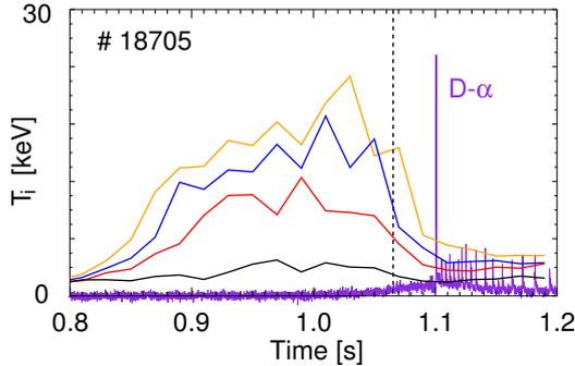
**Figure 2.** Core  $T_i$  measurements from CXRS and ELM timing from D- $\alpha$  divertor signal (violet). Different colours of the  $T_i$  traces correspond to different lines of sight. The dashed line marks the beginning of the ITB loss.
