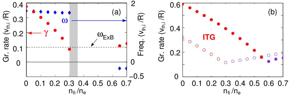
**Figure 3.** GS2 scan of  $n_{fast}/n_e$ . (a) At ITB onset:  $r/a=0.3$ ,  $\hat{s}=0.5$ ,  $\alpha=0.01$ ,  $T_i=7$  keV,  $T_e=3.5$  keV,  $T_{fast}=70$  keV,  $R/L_{T_i}=10$ ,  $R/L_{T_e}=6$ ,  $R/L_{T_{fast}}=0.5$ ,  $R/L_{n_e}=4$ . (b) During the ITB phase:  $R/L_{T_i}=15$ ,  $R/L_{T_e}=7$ , other parameters as in (a). Full points refer to  $T_i/T_e=2$ , empty symbols to  $T_i/T_e=2.5$ . For violet points the ITG is not the leading mode.
