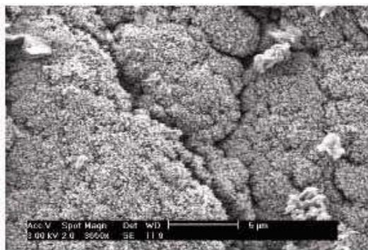
Fig.1. Micrograph of cauliflower-like carbon T-10 film
