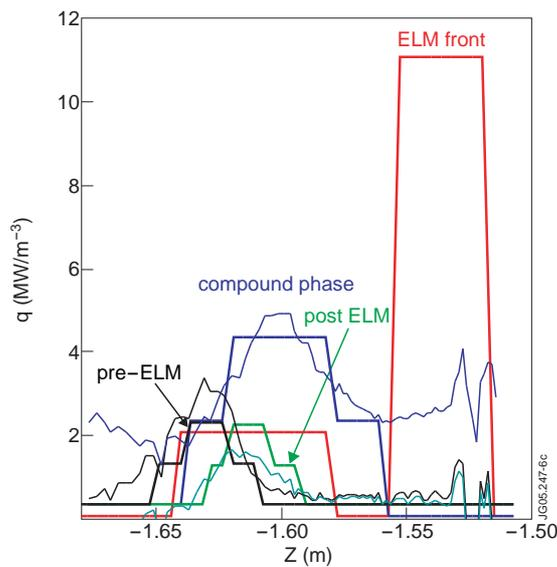
Fig. 3: Profiles of power density on outer divertor during various ELM phases from model (block profiles) and IR data, refer to text.
