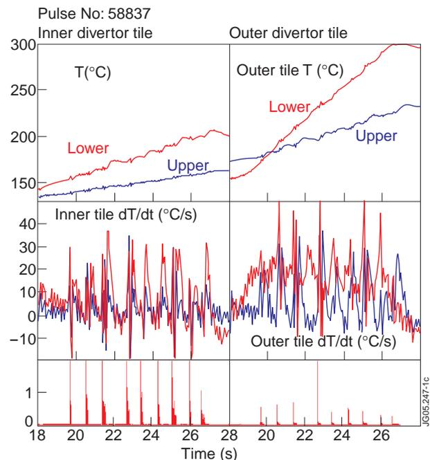
Fig. 1: measurements at inner (left) and outer (right) divertor tiles. Top row: temperature in lower and upper TCs. Middle rows: dT/dt (negative spikes at ELM times due to noise pick-up). Bottom rows:  $D_\alpha$  signals, showing ELM times.
