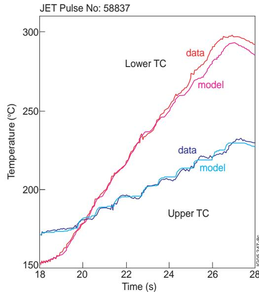
Fig. 6: corresponding measured and simulated  $T$  at TCs.
