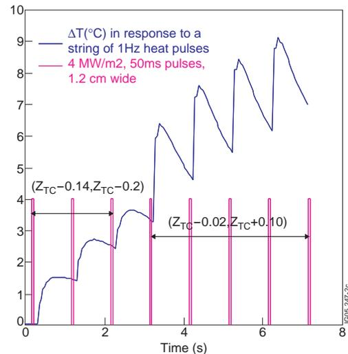
Fig. 2:  $T$  1 cm deep into divertor tile, in response to heat pulse oscillations, placed away or near the TC location
