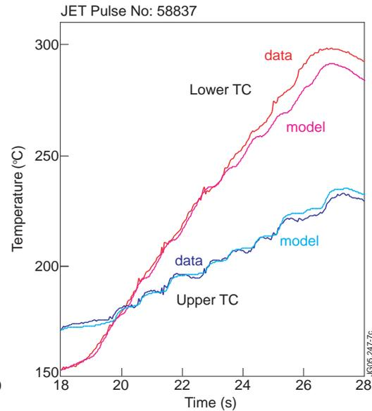
Fig. 4: Measured and modelled  $T$  at TC locations (-1.64 and -1.54 m) from profiles of Fig. 3
