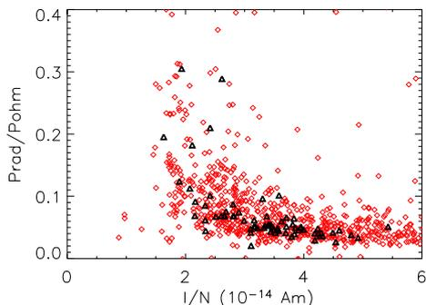
Fig.5 Total radiated power fraction versus I/N for 600KA RFX-mod (black triangles) and RFX discharges (red rhombs).
