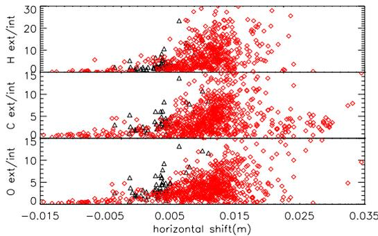
Fig.3 Influx poloidal asymmetry versus plasma horizontal shift, for RFX-mod (black triangles) and for RFX (red rhombs).
