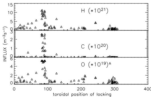
Fig. 4 Hydrogen , carbon and oxygen influxes on a vertical chord, close to the diameter , towards the toroidal position of the locking. For carbon the averaged influx far from the locking is about  $3 \cdot 10^{18} \text{ m}^{-2} \text{ s}^{-1}$
