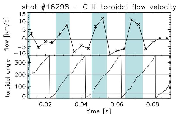
Fig.8 Measured CIII toroidal velocity and toroidal position of the maximum of the external  $m=0$  applied perturbation as functions of time. The green rectangles represent the time intervals during which the maximum of the perturbation is 'seen' by the diagnostic.
