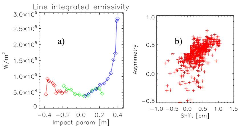
Fig.7 a) Emitted power radial profile. b) Emitted power integrated on external and internal region towards the plasma horizontal shift.
