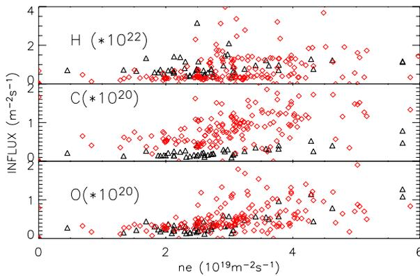
Fig.2 From the top: hydrogen, carbon and oxygen influxes towards plasma density in 600 KA discharges for RFX-mod (black triangles) and for RFX (red rhombs). Influxes are measured on an external chord.
