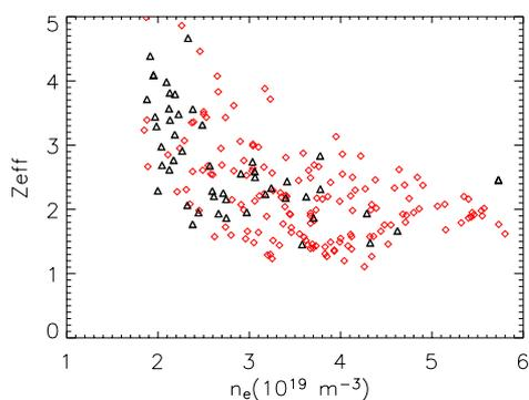
Fig.6 Effective charge measured from visible bremsstrahlung versus electron density for 600KA RFX-mod (black triangles) and RFX discharges (red rhombs).
