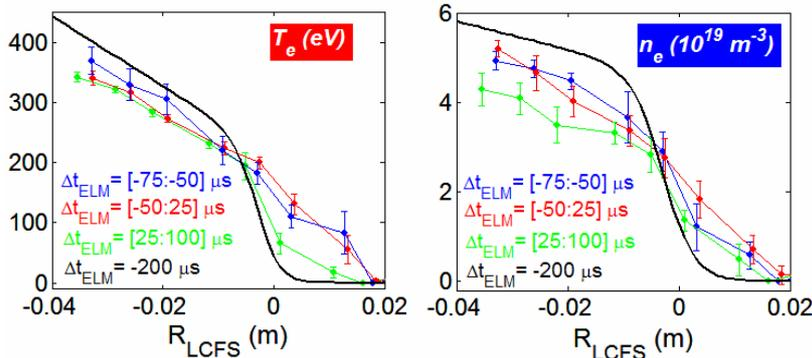
*Fig. 5:* Averaged  $T_e$  and  $n_e$  profiles measured in different time windows during the transient phase ( $\pm 100\mu\text{s}$  from the peak of the ELM signal). A profile fit for  $\Delta t_{ELM} = -200\mu\text{s}$  is shown as reference.
