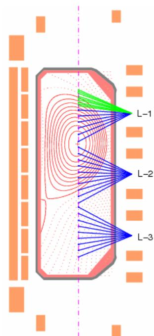
*Fig. 1: TCV poloidal cross section and flux surfaces for shot 26393 at  $t=0.7\text{s}$ . Viewing chords of TS system main (blue) & edge (green).*
