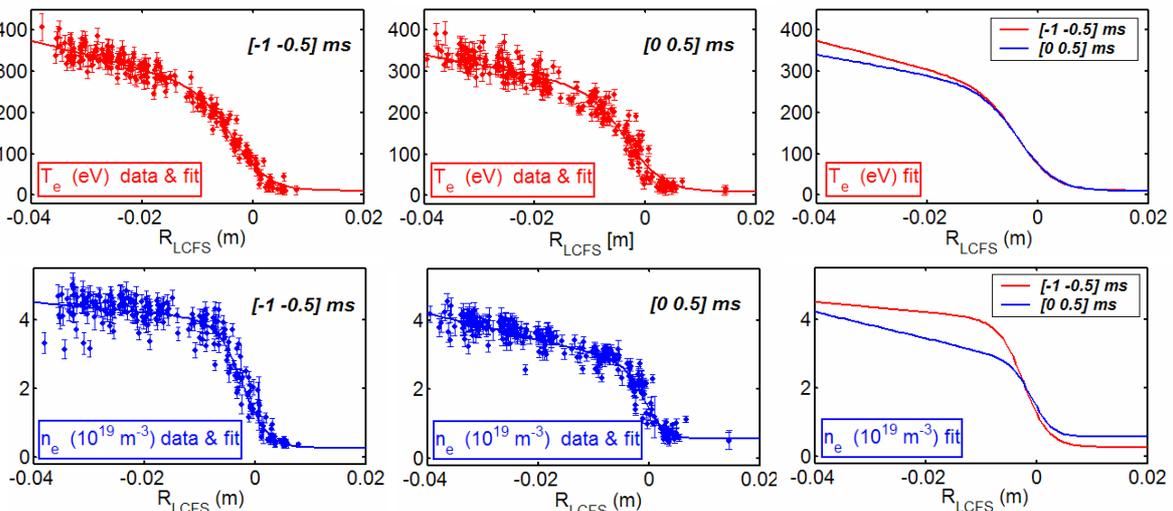
Fig. 2: Results of analysis in bins,  $n_e$  and  $T_e$  profiles data from series of reproducible shots (TCV-# 26387 to 26393) superposed, bin  $[-1, -0.5]$  ms and bin  $[0, +0.5]$  ms delay with respect to ELM.
