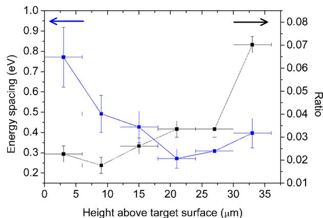
**Figure 3.** Ratio between modulation amplitude and integrated resonance line emission, and spacing between modulations versus height above the target surface.
