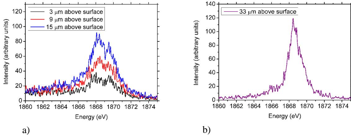
**Figure 2.** Cross-sections of the Al He $\beta$  profile are shown a) close and b) far from the target surface.
