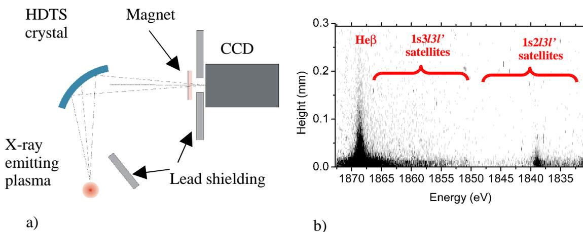
**Figure 1.** a) Experimental geometry and b) a sample of spatially resolved time integrated data.
