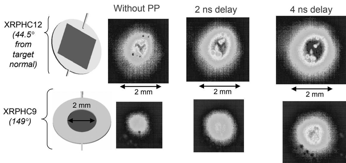
*figure 3 X-ray pinhole images taken from both sides of the target for the case without prepulse and for 2 delays for the heating pulse.*
