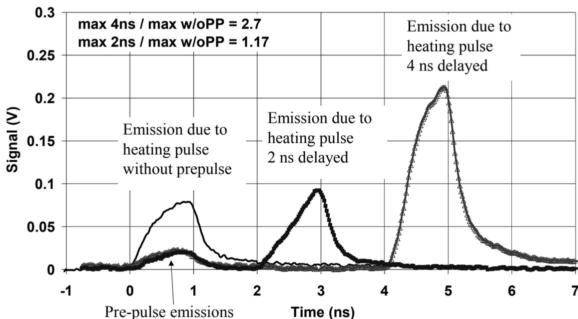
figure 2 Time resolved signals of the DMX Pt channel representative to the multi-keV x-ray emission of germanium produced by the heating laser pulse, delayed in time or not.
