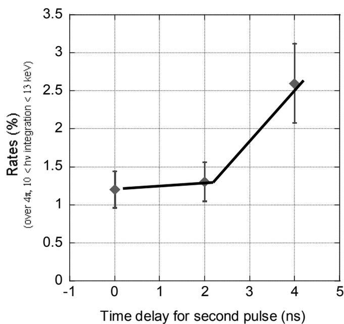
figure 1 Absolute germanium multi-keV X-ray conversion rates obtained with DMX for spatial integration over 4π and photon energies between 10 and 13 keV.
