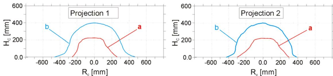
Fig. 2. Crater shapes and dimensions for the disk (a) and direct laser action (b) in two perpendicular projections. The volumes of the craters presented here amount to:  $1.83 \cdot 10^{-5} \text{ cm}^3$  for the disk and  $1.05 \cdot 10^{-4} \text{ cm}^3$  for the direct laser action. The essential differences between the disk produced craters
