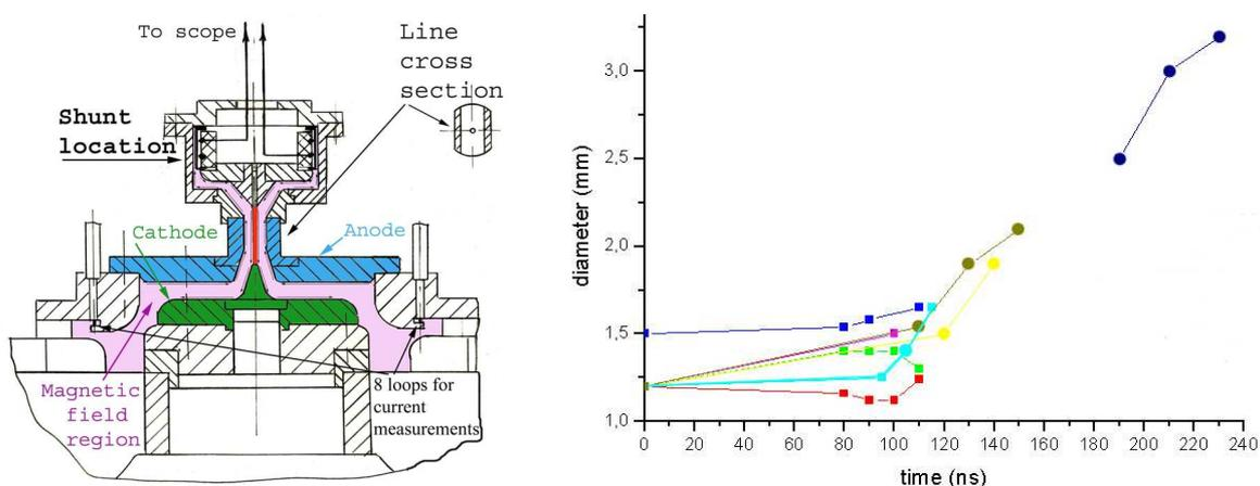
**Fig.1. Left - the scheme of experiment. Right –cathode plasma diameter derived from the shadow and Schlieren images. Lines of proper color join points from the same shot together.**
