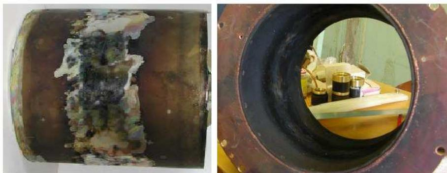
**Fig.6. At the left- stainless steel anode; at the right- carbon-carbon cathode of the POS is shown. The belt erosion region by electron and ion bombardment correspondingly is seen.**
