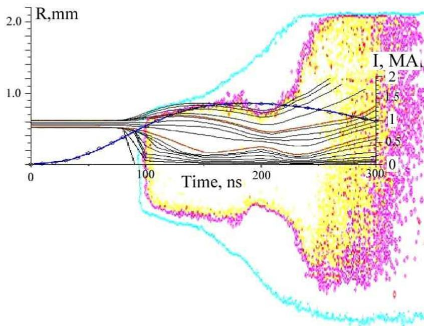
**Fig.2. Superposition of the darkening isolevel lines of the visual light chronogram (sky blue-violet-yellow in the ascending order) with calculated curves (black and brown solid lines). Full blue curve is an electrical current.**
