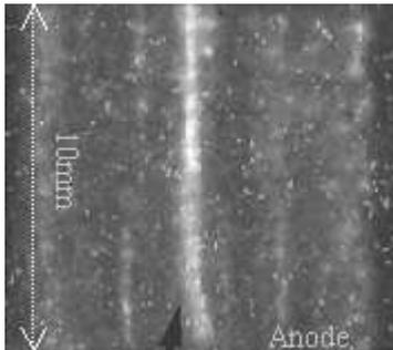
Figure 1. X-ray Frame Image of Single Tungsten Wire Array
