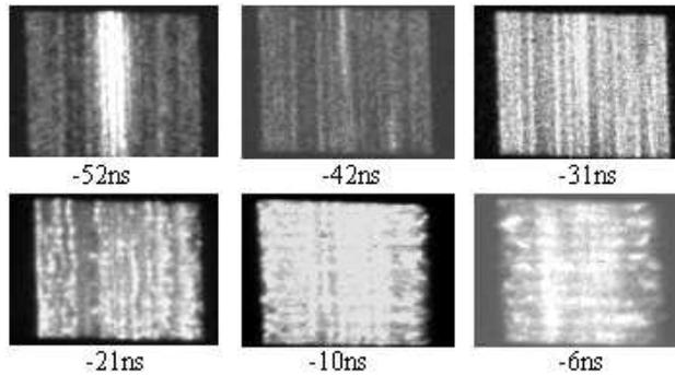
Figure 2. X-ray Multiframe Image of Nested Tungsten Wire Array
