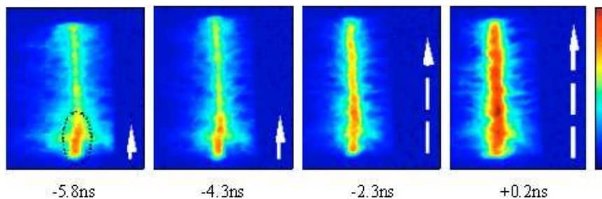
Figure 4 Evolution of hot region for single array consists of 60 wires
