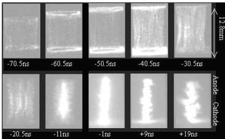
Figure 3. X-ray Multiframe Image of Single Tungsten Wire Array
