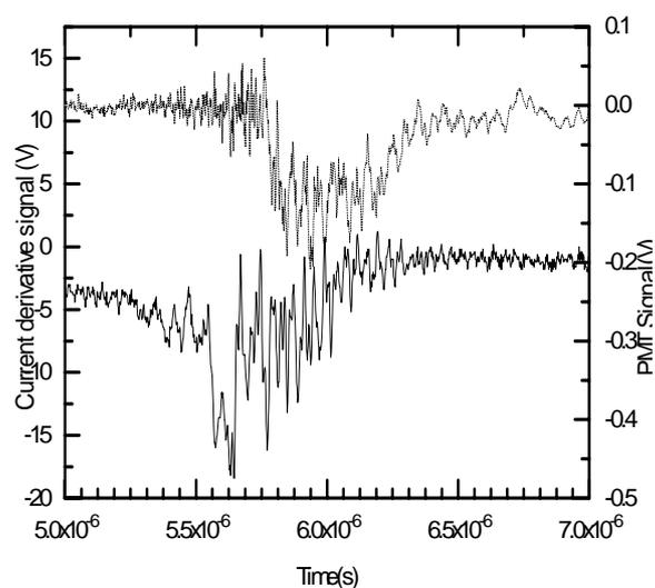
Figure 1. Oscillograms of: PMT signal (upper trace) and current derivative signal (lower trace) for deuterium discharge.
