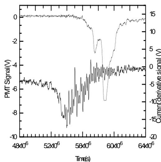
Figure 2. Oscillograms of: PMT signal with hard x-ray filter (upper trace) and current derivative signal (lower trace) for deuterium discharge.
