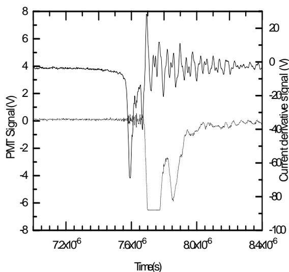
Figure 3. Oscillograms of: Current derivative signal (upper trace) and PMT signal (lower trace) for deuterium+2% krypton discharge.
