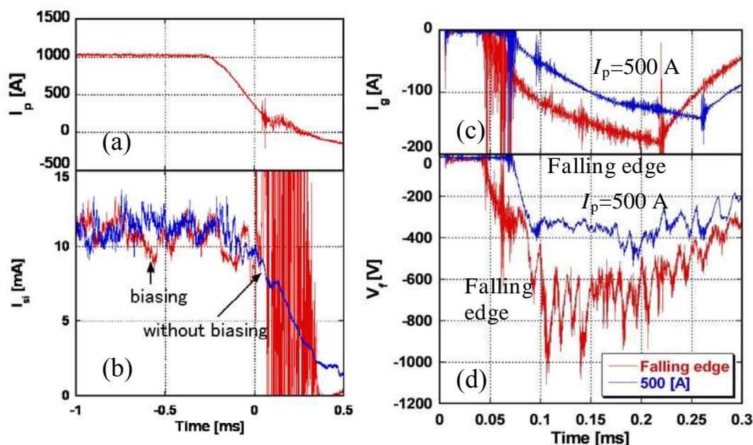
Fig.5. Biasing in the falling edge of plasma current (a) plasma current, (b) ion saturation current, (c) electrode current, (d) floating potential,  $B_T = 0.11$  T.
