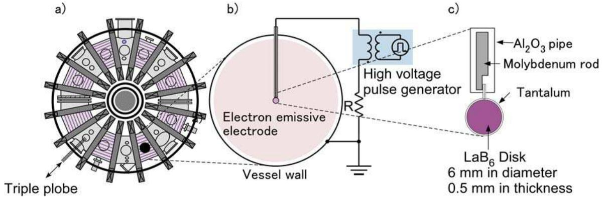
Fig.1. Experimental set up, a) top view of the CSTN-IV, b) biasing circuit, c) configuration of electron emissive electrode.
