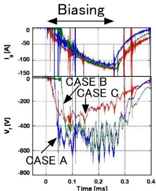
Fig.2. Time evolution of electrode current ( $I_g$ ) and floating potential ( $V_f$ ) at  $r = 0$  cm with plasma current ( $I_p$ ) = 300 A (CASE A), 500 A (CASE B) and 1 kA (CASE C) and toroidal magnetic field ( $B_T$ ) is 0.13 T.
