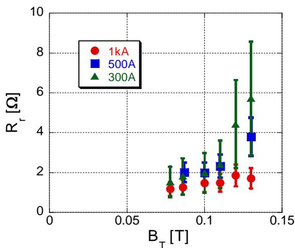
Fig.3. Radial plasma resistance as a function of  $B_T$ .
