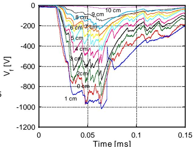
Fig.4. Time evolution of floating potential at the each place measured by probe array.
