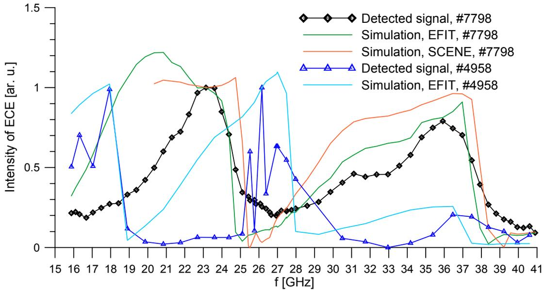
Fig. 2: Comparison of detected and simulated ECE signals, MAST, shots #7798 ( $t=280$  ms) and #4958 ( $t=120$  ms).
