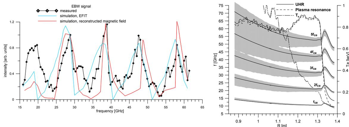
Fig. 3: MAST shot #8694, t=280 ms. Comparison of two simulations (EFIT and reconstructed magnetic field) with experiment (left), reconstructed magnetic field (right).
