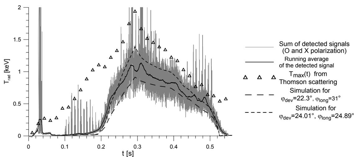
Fig. 4: The time development of EBW signal detected by the NSTX antenna operating at 16.5GHz. Shot #113544.
