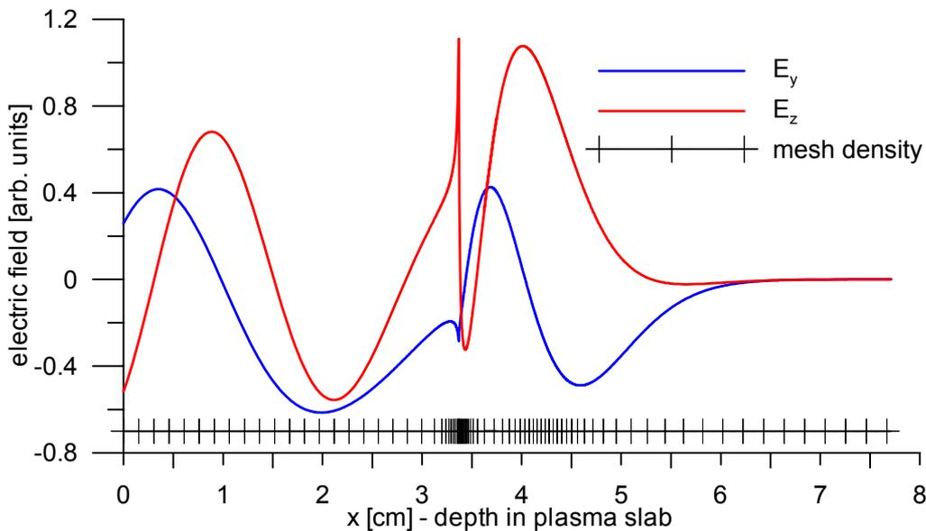
**Fig. 1: Full wave solution in cold plasma slab. NSTX shot #113544,  $t=0.325$  s,  $f=16.5$  GHz.  $x$  axis parallel with the density gradient,  $z$  axis parallel with the magnetic field.**
