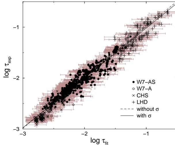
Figure 1: Plot of the confinement time from experiment vs. fit. The dotted line represents the result for the analysis not employing the uncertainties. The error bars are stated for both  $\log \tau_{exp}$  and  $\log \tau_{fit}$ .
