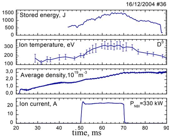
Fig. 3. Evolution of stored energy, ion temperature and averaged density during NBI heating with  $P_{beam}=330kW$ .
