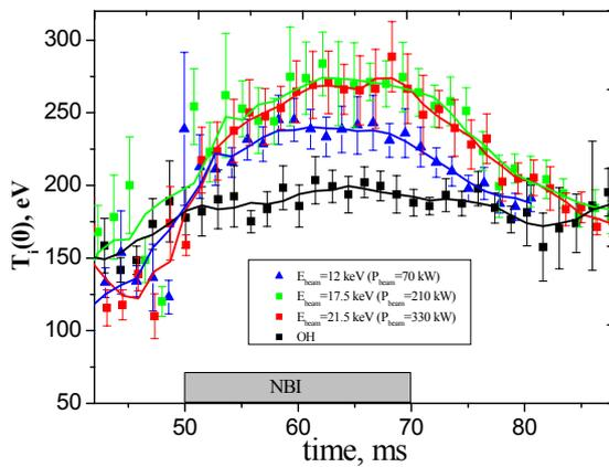
Fig. 4. Dependence of  $T_i(0)$  on power of heating beam.
