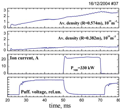
Fig. 1. Evolution of density averaged over vertical chords  $R=0.574m$  (central) and  $R=0.718m$  (outer periphery) during NBI.
