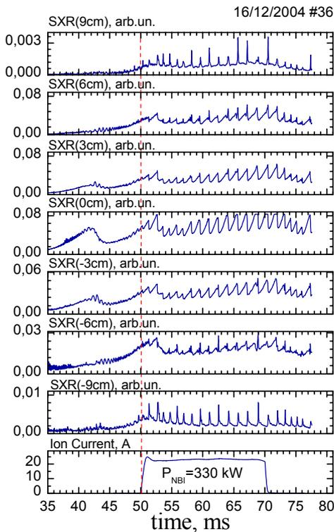
Fig. 2. Intensity of SXR radiation measured along different chords (shift from the center is indicated in brackets). Ion current in the bottom window indicates duration of NBI.
