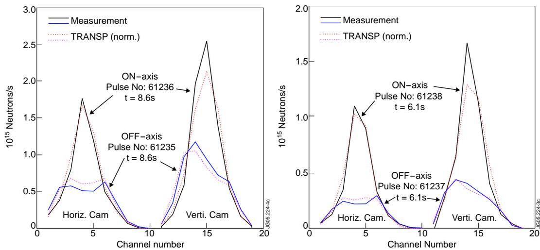
**Figures 3 and 4.** Neutron camera profiles for low power (left) and high power (right) high  $q_{95}$  regime showing on-axis (peaked) and off-axis (flattened) T deposition and comparing simulation with measurement (Bicorn).
