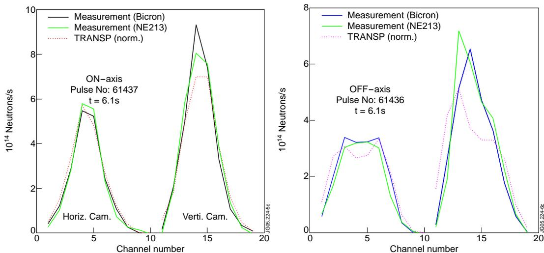
**Figures 5 and 6.** Neutron camera profiles for on-axis (left) and off-axis (right) T beam at low  $q_{95}$  comparing simulation with measurement.
