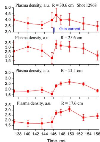
*FIG. 5. Electron density evolution at different spatial points of the plasma column as derived from multi-pulse Thomson scattering diagnostics. The geometric axis of the column is at  $R = 33 \text{ cm}$*
