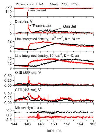
FIG. 4. Waveforms of plasma discharge parameters in Globus-M under plasma and gas jet injection
