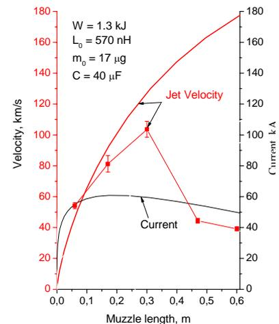
FIG. 1. Evolution of plasma velocity and discharge current distribution along the muzzle length of coaxial electrode accelerator
