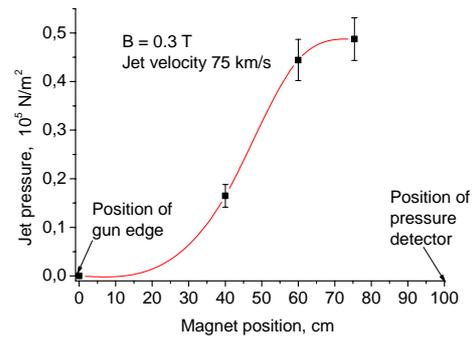
FIG. 3. Plasma jet pressure plotted vs distance between the permanent magnet and the plasma gun edge
