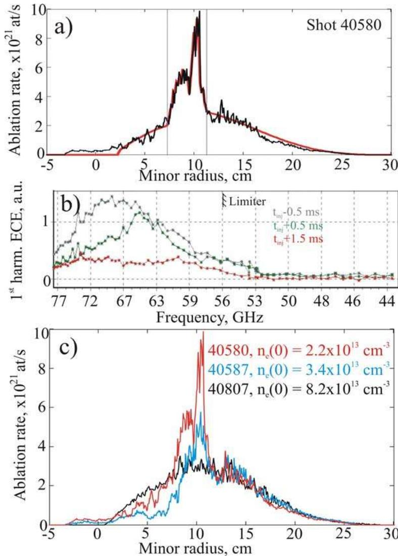
Fig.1 Carbon pellet ablation in T-10 OH mode. a) Experimental and NGS model calculated ablation profiles. b) Evolution of first harmonic ECE spectra during pellet ablation. c) Density scan.
