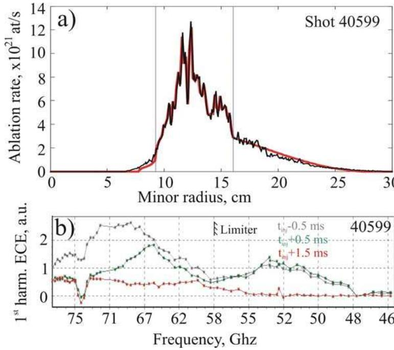
Fig.2 Carbon pellet ablation in T-10 ECRH mode. a) Experimental and NGS model calculated ablation profiles. b) Evolution of first harmonic ECE spectra during pellet ablation.
