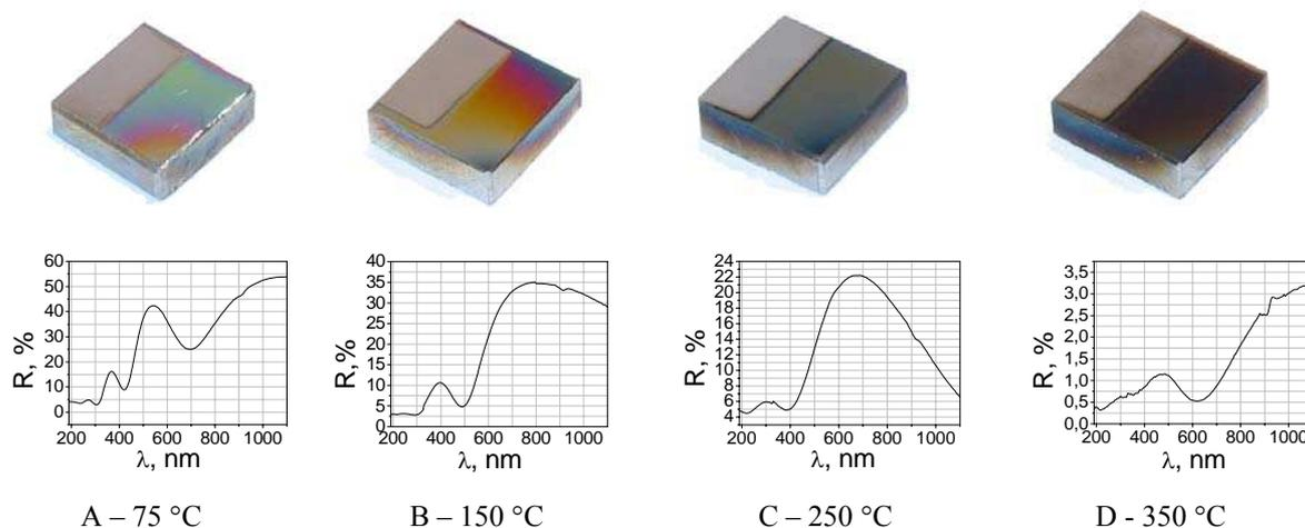
Fig.2. Photos of mirrors and their spectra after magnetron deposition at different temperatures
