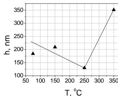
Fig.3. The film thickness depending on the temperature of mirror
