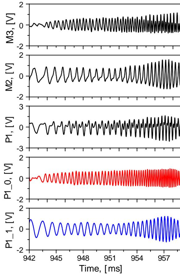
Fig. 2. Cylindrical Fourier harmonics with  $m=3$  (M3) and  $m=2$  (M2); signal of a magnetic probe (P1); P1\_0 and P1\_1 are the components of P1 decomposed by EMD.
