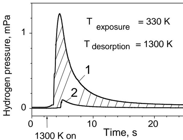
Fig. 1. Hydrogen thermodesorption at permanent pumping with a 200 l/s speed
