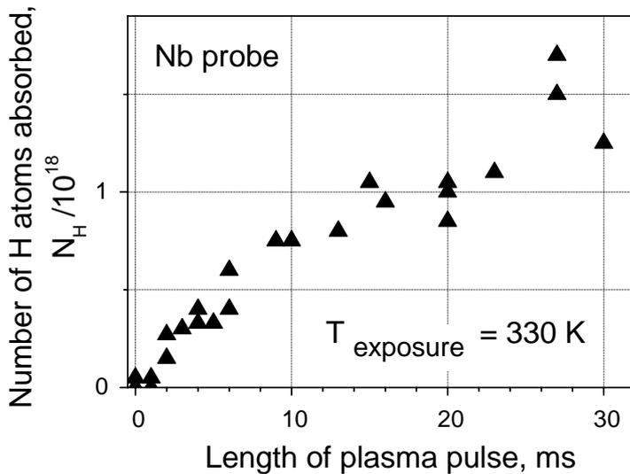
Fig. 3. Dependence of hydrogen absorption on pulse length (suprathermal hydrogen: fig.2 curve 2, left axis). Correspondingly, the fluence of suprathermal hydrogen particles is  $N_H / \alpha_H \times S_{probe} \approx 10^{17} \text{ H/cm}^2$ .
