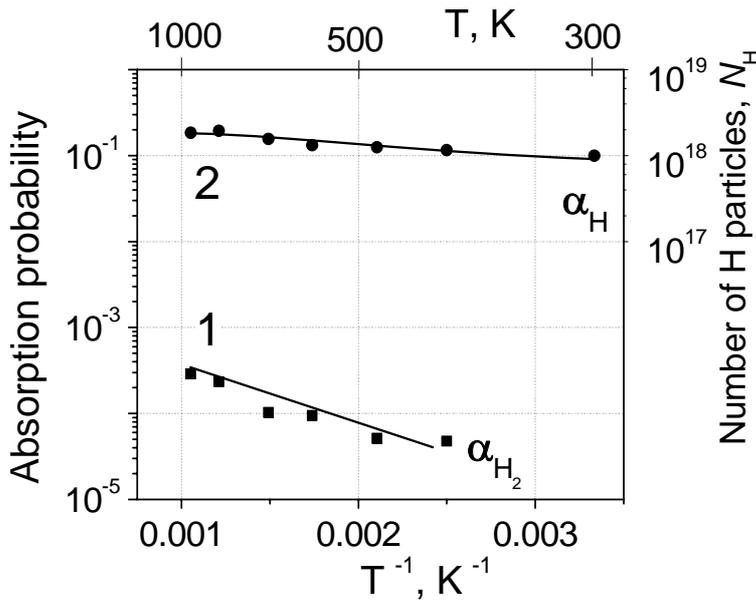
Fig. 2. Temperature dependence of the probability of hydrogen absorption by the probe surface: (1) hydrogen molecules, (2) suprathermal particles (Franck-Condon atoms)
