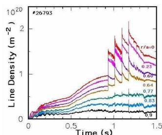
**Fig. 2** Lines integrated measures in a multipellet discharge 26793.
