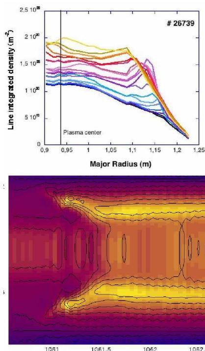
**Fig. 4** Profiles during pellet ablation. a): Density line integrated profiles; b): Density contour plot.
