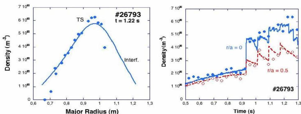
Fig. 3 timing density evolution, the blue line is the measure by Thomson scattering
