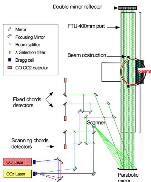
**Fig. 1** Scanning interferometer schematic view: an oscillating mirror scans the beam.
