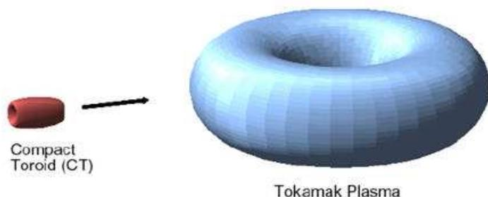
Figure 1: Pictorial representation of CT Fuelling. The CT velocity is about 300km/s. Other relevant time scales are: CT penetration time of a few micro-seconds, CT dissipation time inside the tokamak of about 100 microseconds and density equilibration time of  $> 1ms$ .
