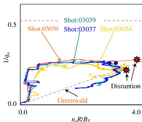
Fig.1. Discharge trajectories, w/o disruption discharges on Hugill diagram. The red star symbols denote the place of disruption occurrence, and the blue solid circles indicate disruption free discharges.
