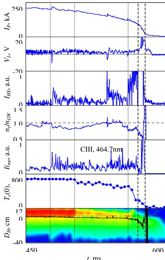
Fig.4. The evolutions during disruption. From the top down, are the plasma current, loop voltage, intensity of hard X ray radiation, ratio between plasma density and Greenwald density limit  $n_e/n_{GW}$ , impurity emission, central electron temperature, horizontal plasma displacement  $D_H$  (with black trace) and the profile of electron temperature which is presented by an image, respectively.
