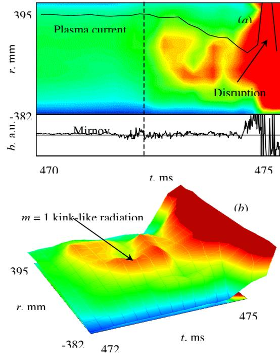
Fig.3. Evolutions of plasma radiation at disruption. *a)* are the waveforms of plasma current (the black trace), image of plasma radiation, and MHD perturbation  $\tilde{b}$ . *b)* is the 3-D representation of plasma radiation.
