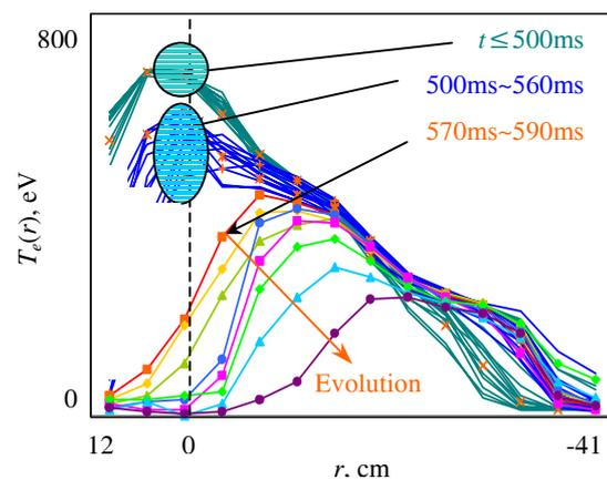
Fig.5. Temporal evolution of the electron temperature profile  $T_e(r)$  during disruption.
