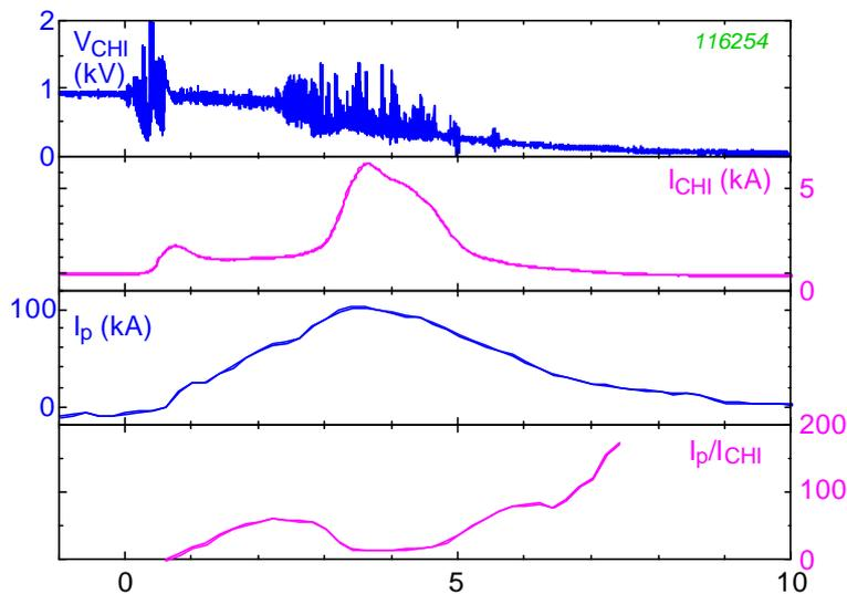
Figure 2: Recent Transient CHI discharge in NSTX. Shown are from top to bottom, the voltage across the injector (lower divertor) electrodes, the injector current, CHI produced toroidal current and the ratio of the toroidal current to the injector current. Note that the current multiplication increases as the injector current decreases, and reached values of up to 170.
