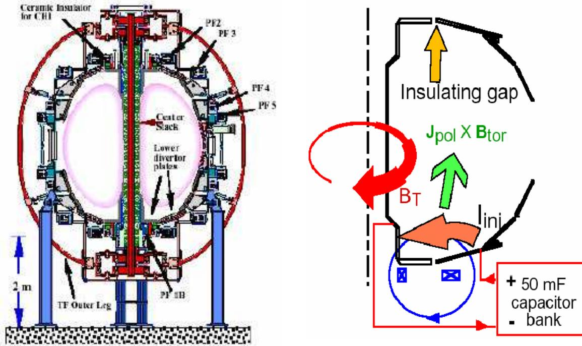
Figure 1: The NSTX Machine layout showing the locations of the upper and lower insulator rings which allow the inner divertor plates and center stack to be biased with respect to the outer components. Figure on the right shows how CHI is implemented in NSTX.
